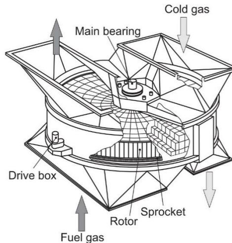
*Sketch of a Ljungström regenerator (rotary heat exchanger) to preheat combustion air with combustion flue gases. Source: Walter and Epple, Numerical simulation of power plants and firing systems (2017)*
